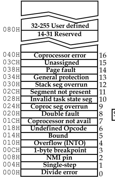
The interrupt vector table is located in the first 1024 bytes of memory at addresses 000000H through 0003FFH.
