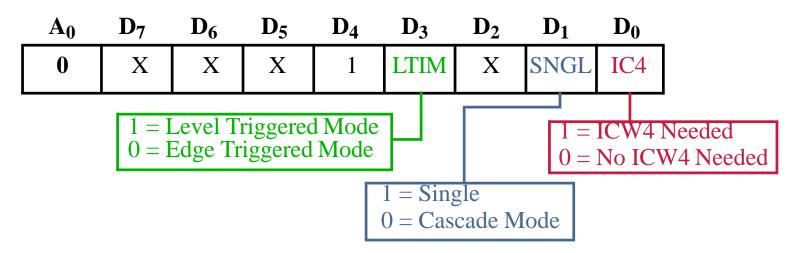
LTIM indicates if IRQ lines are positive edge-triggered or level-triggered.
