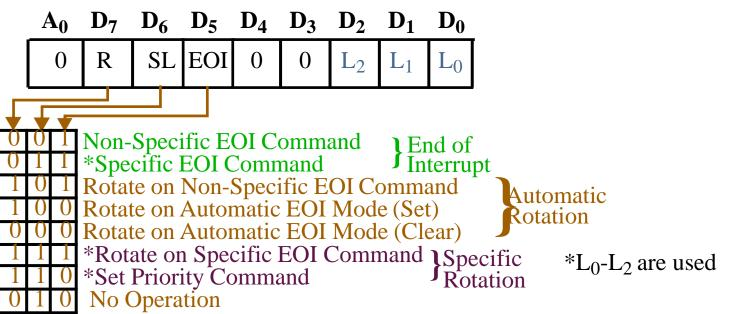
*Non-specific EOI*: Here, the ISR sets this bit to indicate EOI. The 8259A automatically determines which interrupt was active and re-enables it and lower priority interrupts.
