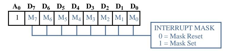
OCW1 is used to read or set the interrupt mask register.
