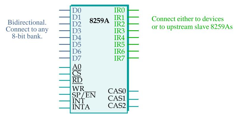
$\overline{\text{CS}}$  and  $\overline{\text{WR}}$  must be decoded. Other connections are direct to microprocessor.
