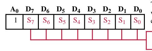
This register is treated as a mask, with 1's indicating the IRQ channels connected to master/slave 8259As.
