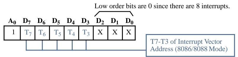
These bits determine the vector numbers used with the IRQ inputs. For example, if programmed to generate vectors 08H-0FH, 08H is placed into these bit positions.
