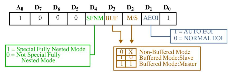
Fully nested mode allows the highest-priority interrupt request from a slave to be recognized by the master while it is processing another interrupt from a slave.
