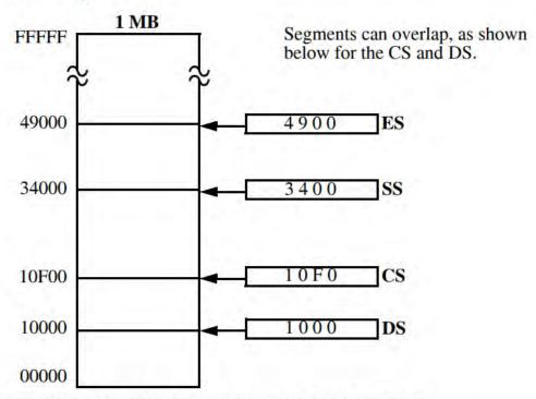
Segmented addressing allows relocation of data and code.
