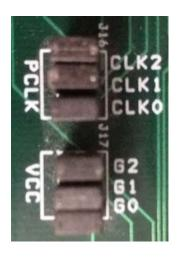
Jumpers for Gate pins short out to VCC.
